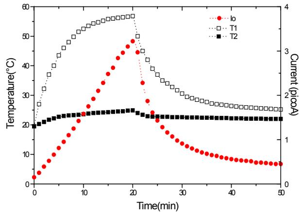
Figure 7 : Temperatures and current collected with an electrode. Flow rate 288 l/h
