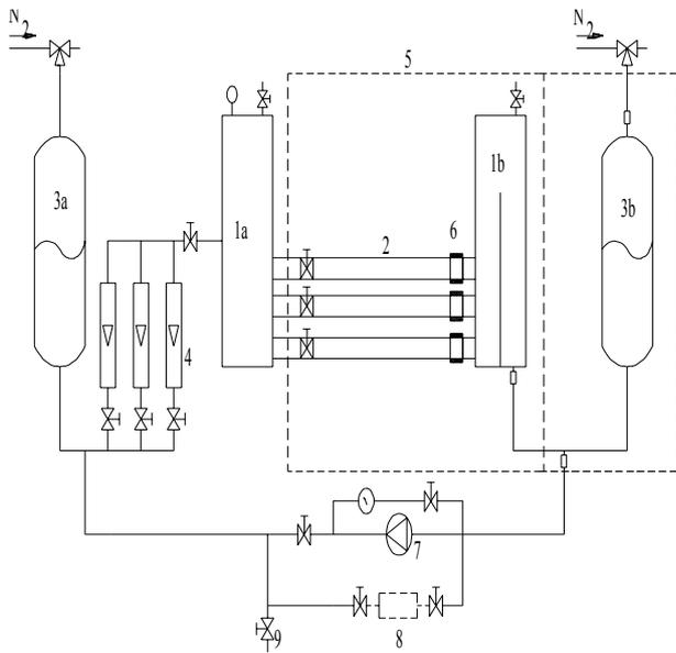
1 Stainless steel vessel, 2 Channels, 3 Vessels under pressure, 4 Flowmeter, 5 Faraday cage, 6 Insulators, 7 Adjustable Pump, 8 Conductivity measurement system, 9 Oil sampler.
