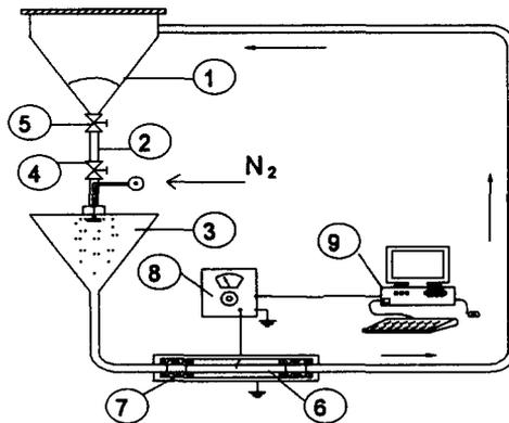
Figure 6 : Pneumatic conveyor experimental equipment.
