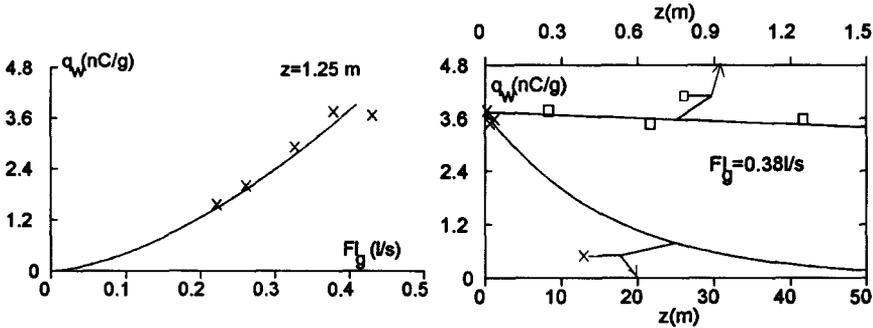
Figure 7 : Charge transferred in terms of flow.
