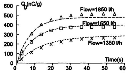
Fig. 5. Charge generated for different flows
