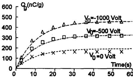
Fig. 4. Charge generated for different voltage
