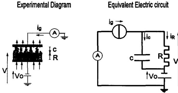
Figure 1. Schematic diagram and equivalent electric circuit diagram.
