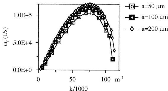
Fig. 7. Growth rate vs. wave number. Influence of the radius of the jet.
