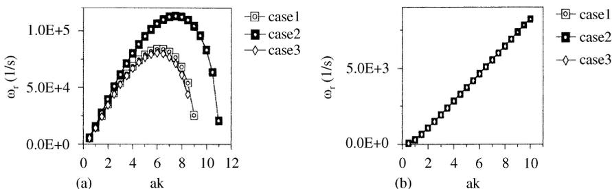
Fig. 2. (a) Influence of the electrification on the real part of the growth rate; (b) Influence of the electrification on the imaginary part of the growth rate.
