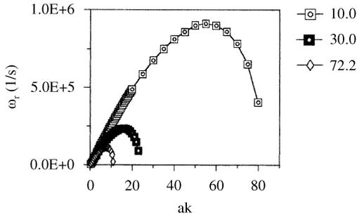
Fig. 6. Growth rate vs.  $ak$  for different values of the surface tension (mN/m).
