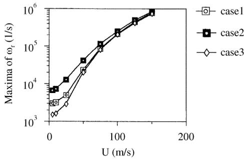
Fig. 9. Influence of the velocity on the maxima of the real part of the growth rate.
