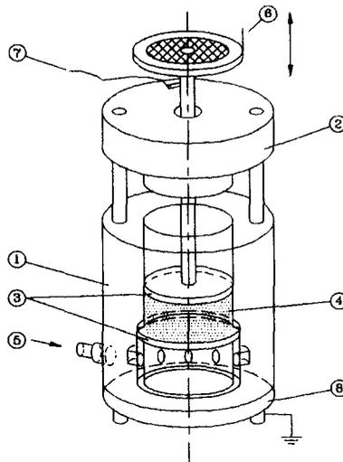
Figure 1. Cell of Measurement: ① Body in Teflon, ② Guide with ball bearing, ③ Porous electrode, ④ Powder, ⑤ Inlet of air flow, ⑥ Support for weight application, ⑦ Voltage supply connection, ⑧ grounded metallic support connected to the chamber and the lower electrode.
