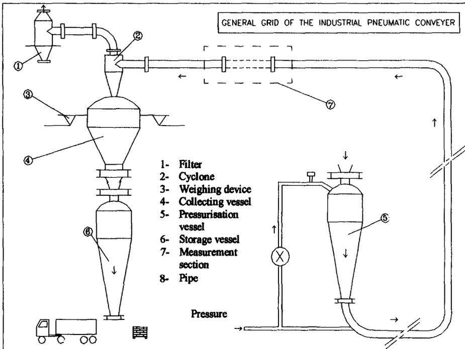
Figure 5. Industrial Set up
