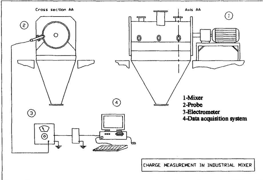
Figure 4. Experimental set up for measurements in the mixer
