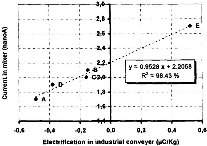
Figure 11. Correlation of pneumatic conveyor and mixer experiment
