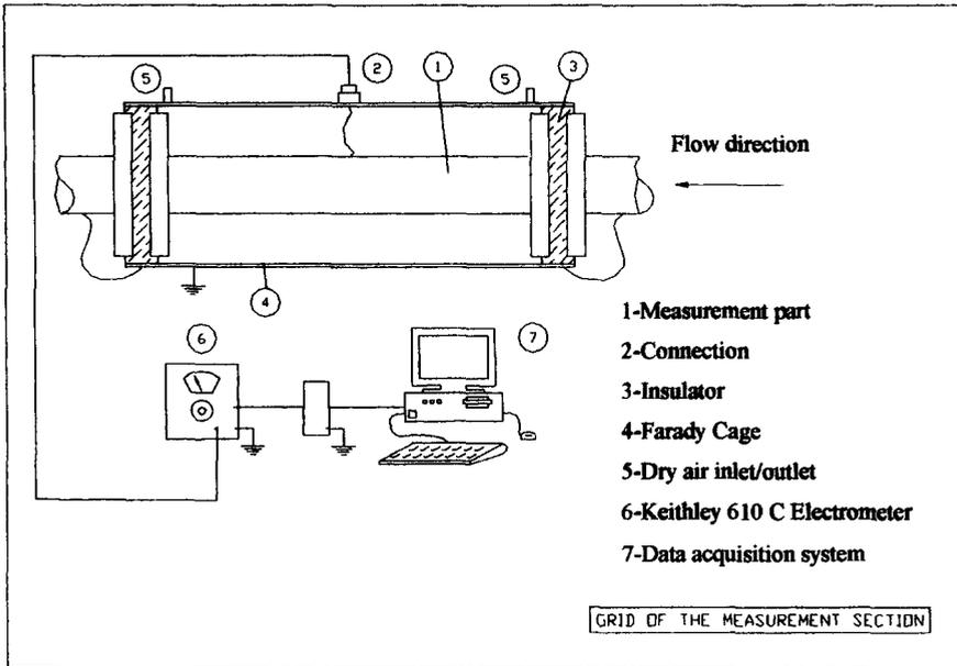
Figure 6. Device for flow electrification measurements
