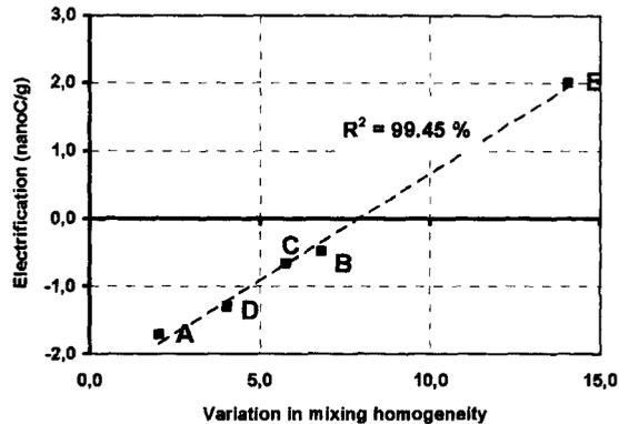
Figure 12. Correlation of flow electrification and variation in mixing homogeneity
