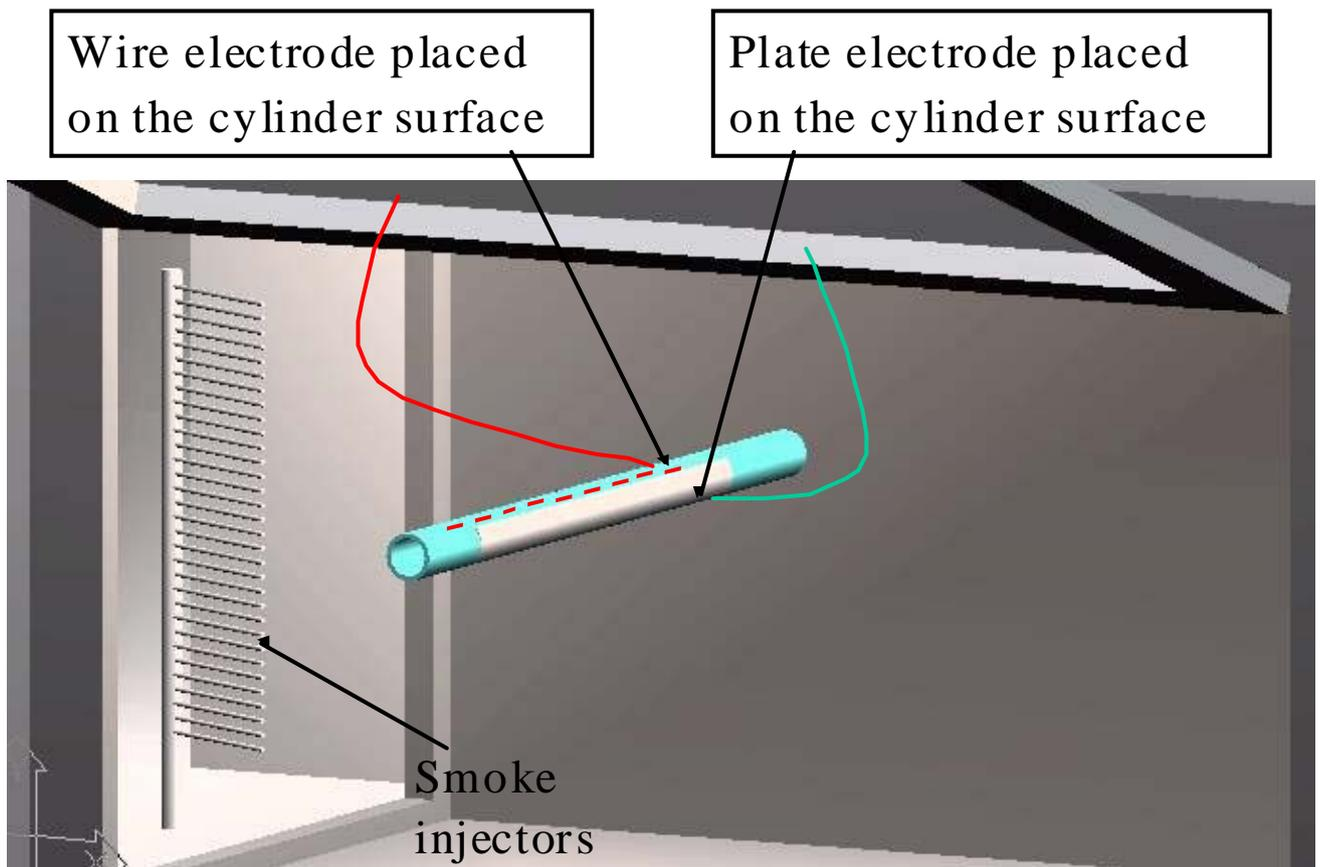
Figure 1: Experimental device: Cylinder placed on a wind tunnel (section 450x450mm)
