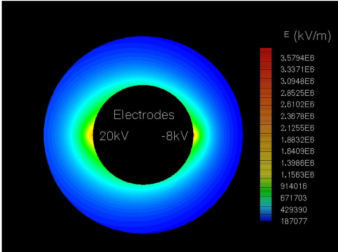
Figure 7: Electric field configuration for a cylinder with a 30 mm diameter
