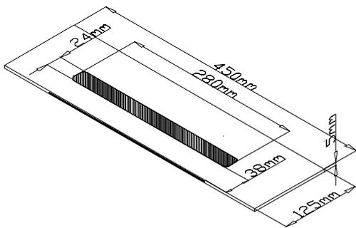
Figure 1 Electrode arrangement
