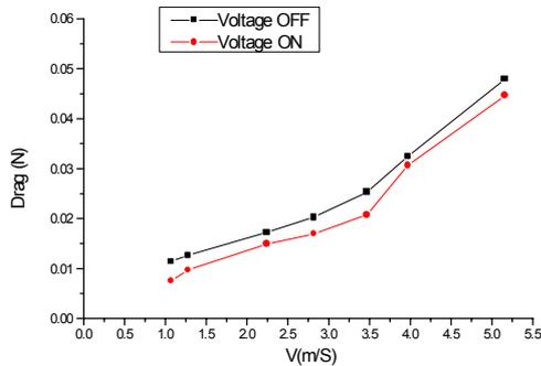
Figure 6: Drag force on one plate surface as a function of flow velocity. ( $\Delta V=33\text{kV}$ ,  $900\mu\text{A/m}$ )
