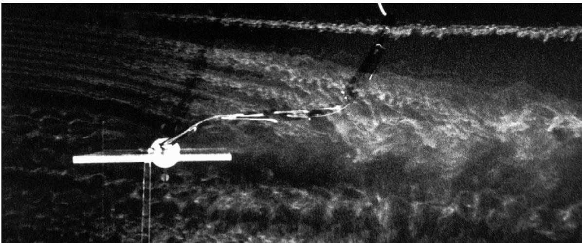
Figure 5b: Flow Visualisation: Voltage on ( $\Delta V = 32 \text{ kV}$ ,  $715 \mu\text{A/m}$ )
