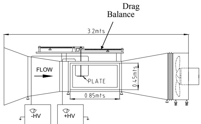
Figure 3: Schema of the wind tunnel
