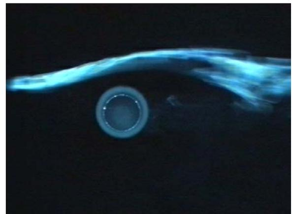
Figures 7: Sequence of visualizations when applying the electric field at time  $T=0.00s$ .  $U_0=0.7m/s$ .  $\Delta\phi=32kV$
