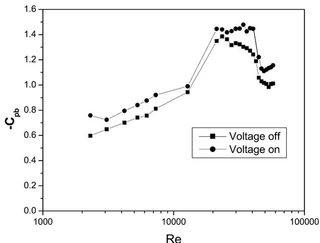
Fig. 10. Base suction coefficient versus Reynolds number, EHD actuator off (squares) and on (circles),  $\Delta V=34$  kV
