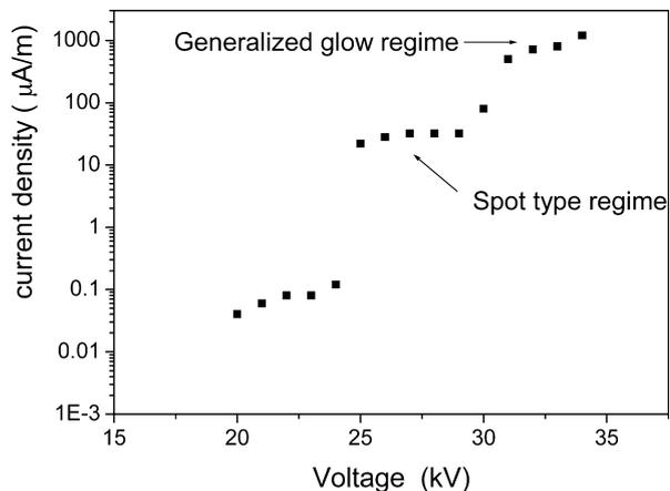
Fig. 3. Voltage versus current per unit electrode length
