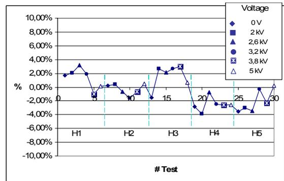
Figure 4 Error of the optical system on flow rate measurement. Tests at different liquid column height (Hi) and electrode Voltage.
