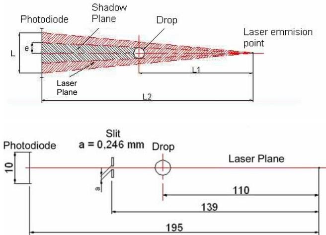
Figure 2: Details of droplet measurement system
