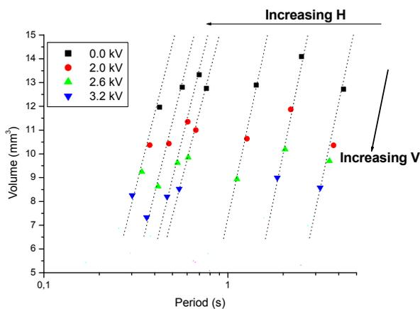
Figure 7: Volume of the droplets as a function of dripping period for different voltages. Dotted lines correspond to constant liquid column height.
