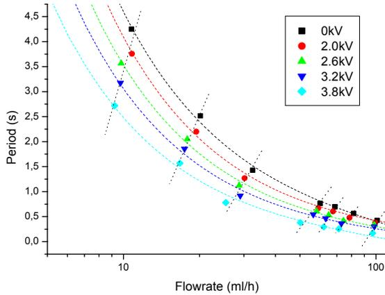
Figure 5: Dripping period as a function of flowrate: Continuous lines are the fitting of the experimental data with Scheele expression. Dashed line links results obtained at the same liquid columns height but at different voltages.
