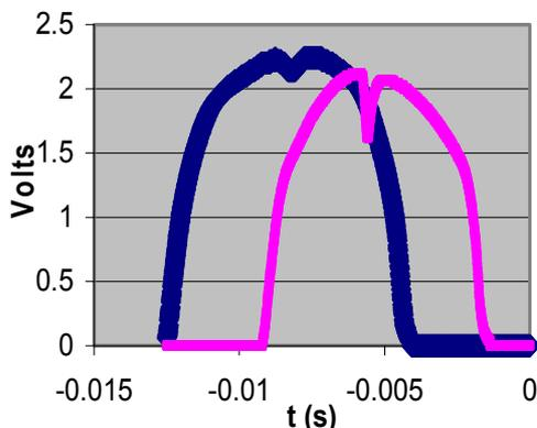
Figure 3: Signals obtained from the shadow of the flying droplet on the photodiodes
