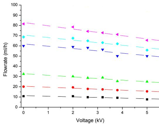
Figure 6: Flow rate variations as a function of applied voltage for fixed liquid column heights (dotted lines)
