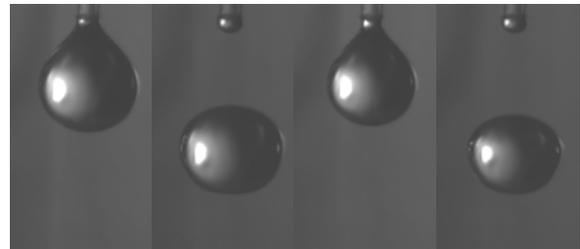
Figure 1 Photography of detaching droplets (V=0 kV left, V=4.0kV right)
