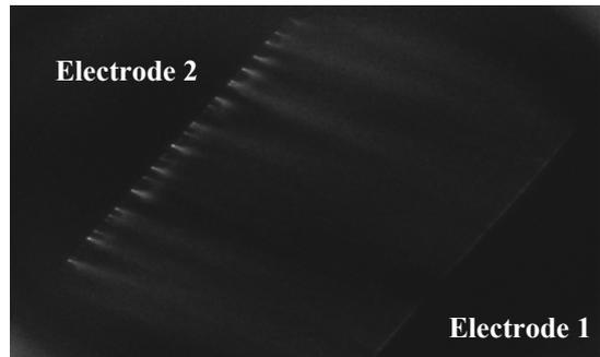
Figure 9 CCD image for an air plasma sheet filtered with a 391.4 nm interferential filter.
