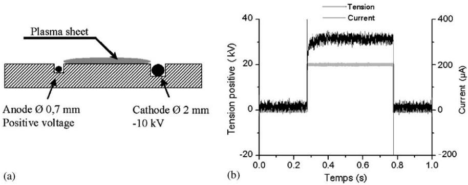
Fig. 1. (a) Schematic side view of the DC surface corona discharge set-up; (b) typical behaviour of the discharge current with a square wave excitation.
