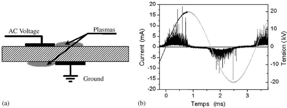
Fig. 2. (a) Schematic side view of the AC surface barrier discharge set-up; (b) typical behaviour of the barrier discharge current.
