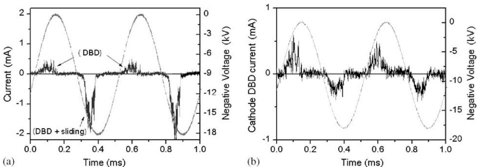
Fig. 4. (a) Typical behaviour of the sliding discharge current when the capacitive component is removed; (b) typical behaviour of the current when the upper negative electrode is removed.
