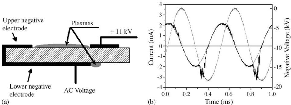
Fig. 3. (a) Schematic side view of the sliding discharge set-up; (b) typical behaviour of current in black and associated voltage in grey for a frequency = 1 kHz.
