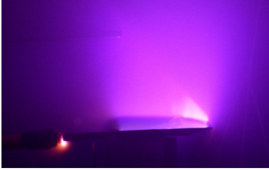
Figure 3. DC discharge on supersonic rarefied air flow over the flat plate.
