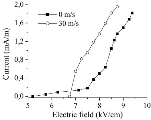
**Figure 6.** Current versus electric field for 2 air stream velocity values.
