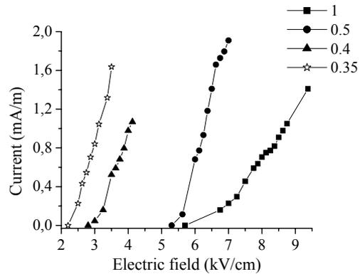
**Figure 11.** Current versus electric field for different air pressure values (in  $10^5 \text{ Pa}$ ).
