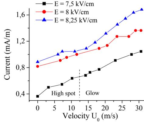
**Figure 7.** Current versus air stream velocity for 3 electric field values.
