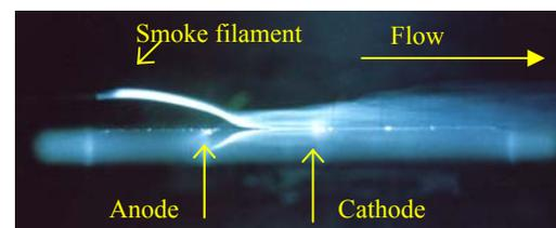
**Figure 2.** Visualisation of an airflow along a flat plate turned off toward the wall by a DC discharge.
