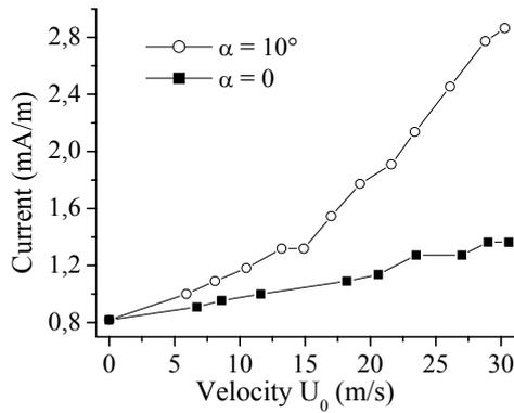
**Figure 9.** Current versus free air stream velocity for  $E = 8 \text{ kV/cm}$ .
