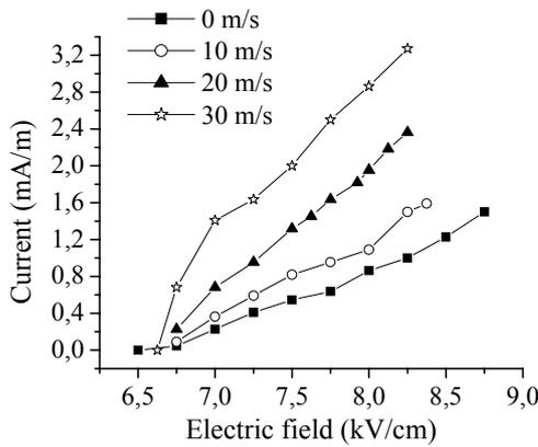
**Figure 8.** Current versus electric field for 4 airstream velocities with  $\alpha = 10^\circ$ .
