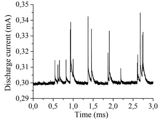
**Figure 5.** Discharge current versus time ( $U_0=0$  m/s and  $E = 7.6$  kV/cm).
