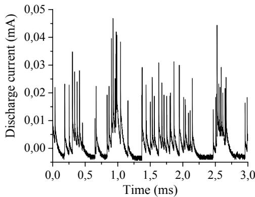
**Figure 10.** Alternating component of the current ( $I_{\text{mean}} \approx 300 \mu\text{A}$ ) versus time for  $U_0 = 30 \text{ m/s}$  and  $\alpha = 10^\circ$ .
