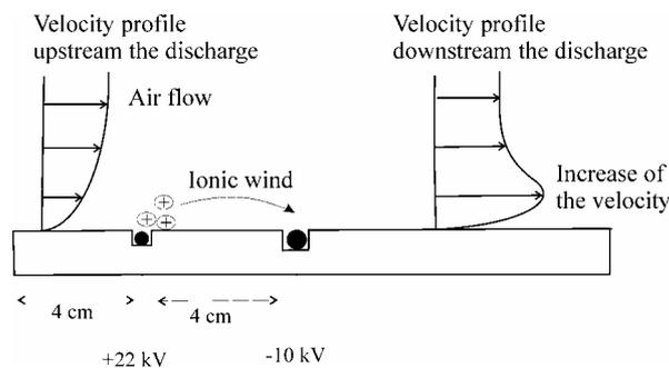
**Figure 1.** Schematic representation of the electrohydrodynamic actuator.
