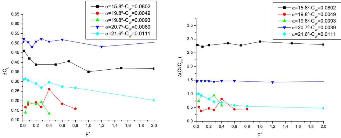
For the case with the lowest angle of attack ( $\alpha=15.8^\circ$ ) an important increase of the aerodynamic coefficients  $C_l$  and of the ratio  $C_l/C_{Dp}$  has observed, as a consequence of actuation. These enhancement was associated, as previously detailed, to the passage from a fully separated flow (actuator off) to a fully attached flow (actuator on).
