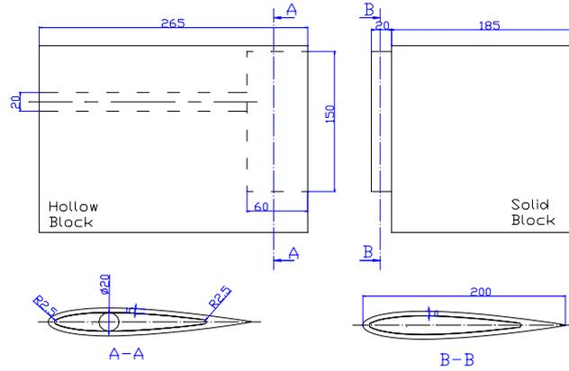
**Figure 1: Scheme of the NACA0015 Airfoil Model.**
