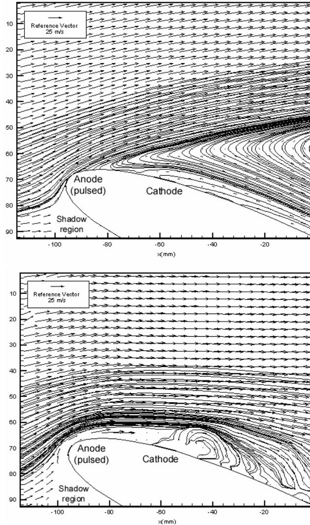
**Figure 9: Middle Post stall Regime Time averaged flow fields with associated streamlines.**
