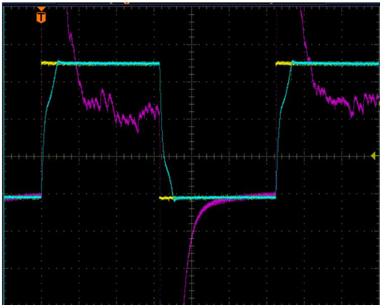
**Figure 2: Discharge current and anode voltage potential waveform at  $f_{exc}$  400Hz**
