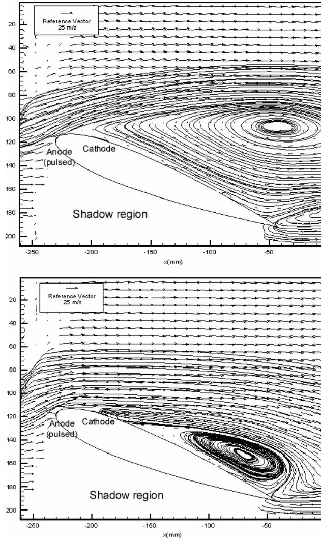
**Figure 11: Deep Post stall Regime Time averaged flow fields and associated streamlines.**
