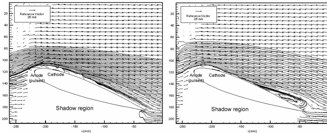
**Figure 7: Near Post stall Regime Time averaged flow fields with associated streamlines.**
