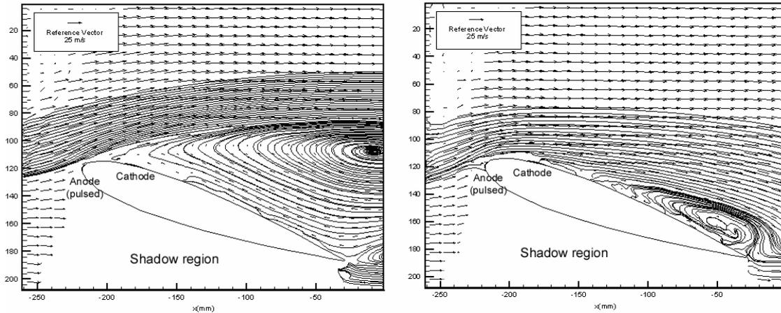
**Figure 6 : Near Post stall Regime Time averaged flow fields with associated streamlines.**
