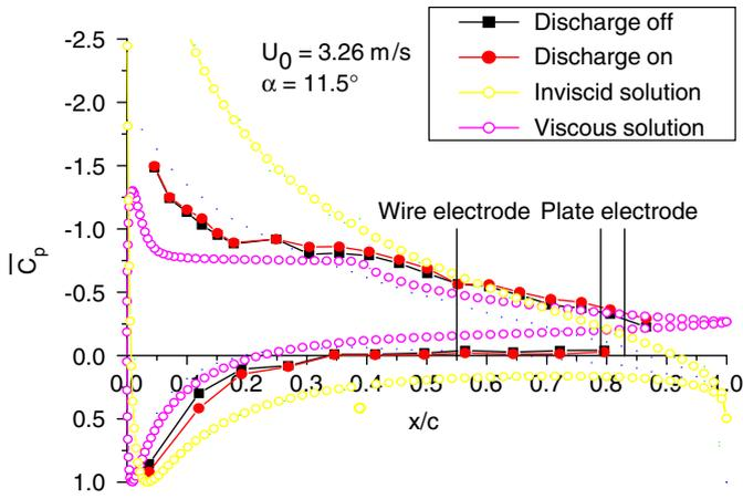
Fig. 9. Dimensionless pressure distribution ( $Re = 43.466$ ,  $\alpha = 11.5^\circ$ ,  $\Delta V = 30$  kV,  $I = 250$   $\mu$ A). Upstream electrode positive.
