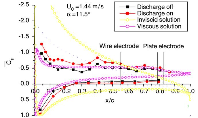
Fig. 7. Dimensionless pressure distribution ( $Re = 19,200$ ,  $\alpha = 11.5^\circ$ ,  $\Delta V = 30$  kV,  $I = 250$   $\mu$ A). Upstream electrode positive.
