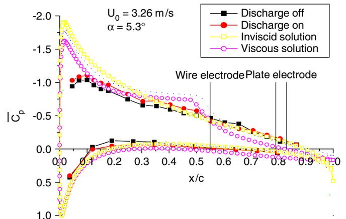
Fig. 8. Dimensionless pressure distribution ( $Re = 43,466$ ,  $\alpha = 5.3^\circ$ ,  $\Delta V = 30$  kV,  $I = 250$   $\mu$ A). Upstream electrode positive.
