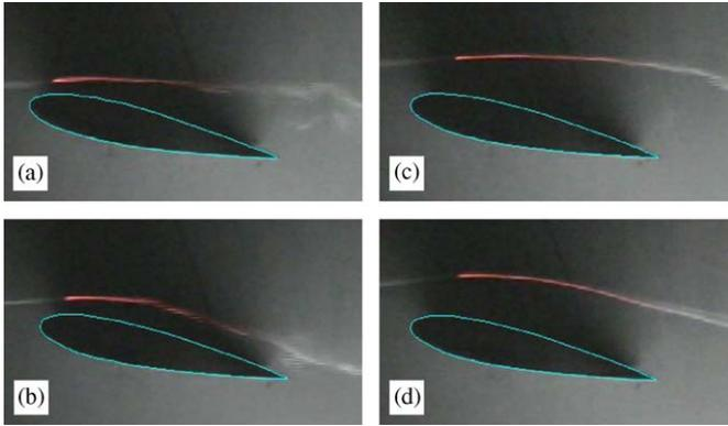
Fig. 6. Flow visualization with two different heights for the smoke filament ( $Re = 15,000$ ,  $\alpha = 11.7^\circ$ ,  $\Delta V = 30$  kV,  $I = 250$   $\mu$ A). Upstream electrode positive. Height 1: (a) discharge off and (b) discharge on. Height 2: (c) discharge off and (d) discharge on.
