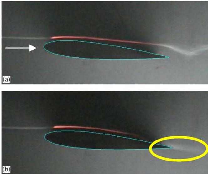
Fig. 3. Flow visualization ( $Re = 15,000$ ,  $\alpha = 5.8^\circ$ ,  $\Delta V = 30$  kV,  $I = 250$   $\mu$ A). Upstream electrode positive. (a) (top) Discharge off, (b) (bottom) discharge on.
