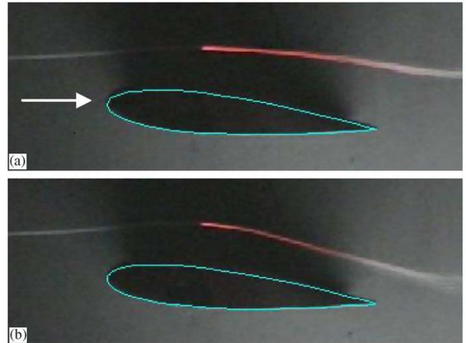
Fig. 4. Flow visualization ( $Re = 15,000$ ,  $\alpha = 5.8^\circ$ ,  $\Delta V = 30$  kV,  $I = 250$   $\mu$ A). Upstream electrode positive. (a) (top) Discharge off, (b) (bottom) discharge on.
