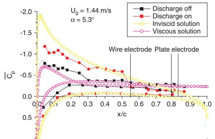
Fig. 5. Dimensionless pressure distribution ( $Re = 19,200$ ,  $\alpha = 5.3^\circ$ ,  $\Delta V = 30$  kV,  $I = 250$   $\mu$ A). Upstream electrode positive.
