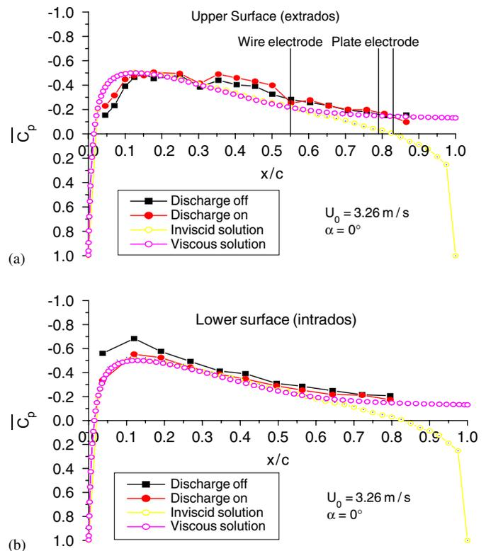
Fig. 2. Dimensionless pressure distribution ( $Re = 43.466$ ,  $\alpha = 0^\circ$ ,  $\Delta V = 30$  kV,  $I = 250$   $\mu$ A). Upstream electrode positive. (a) (top) Upper surface, (b) (bottom) lower surface.
